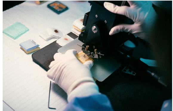
Figure 6.10 In the preparation stage of making the TMA at the arrayer the bridge is placed over the recipient block.
