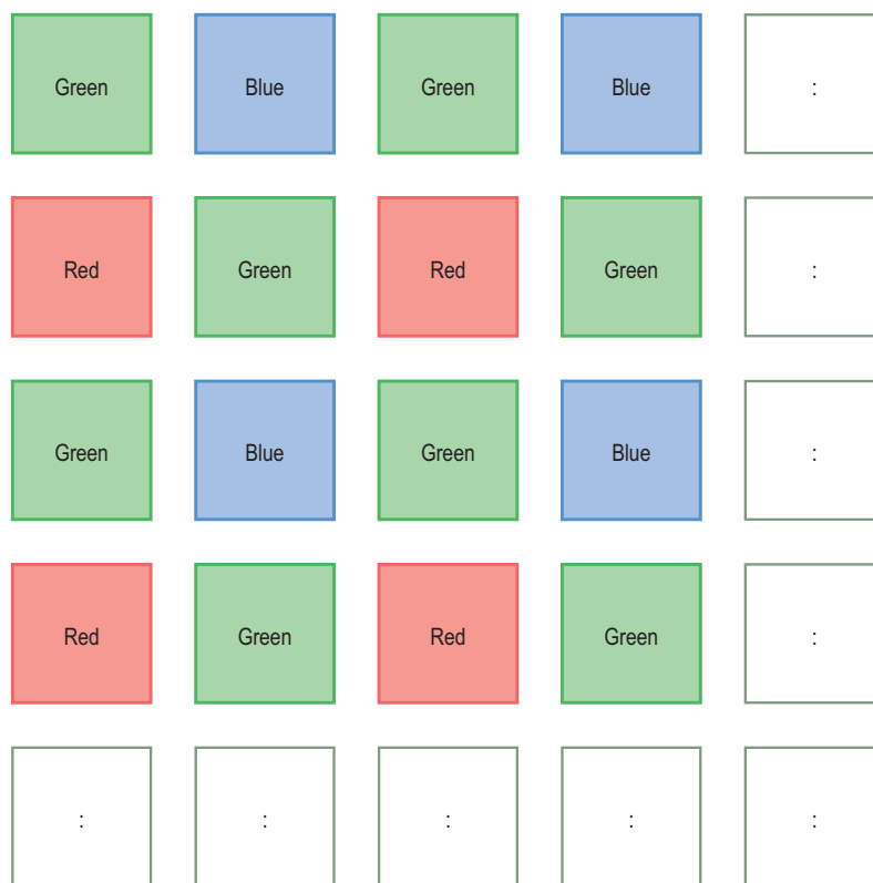
Figure 23.1 The Bayer pattern of color filters applied to individual pixels of single-chip color cameras. Note that this effectively reduces the color resolution of the chip to one-fourth that of the true number of pixels.
