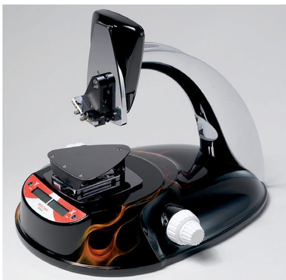
Figure 6.7 Manual tissue arrayer MTAII, manufactured by Beecher Instruments, Inc.
