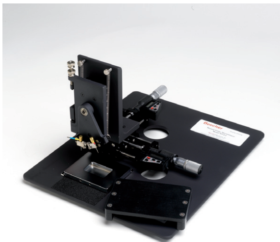
Figure 6.6 Manual tissue arrayer MTAI, manufactured by Beecher Instruments, Inc.
